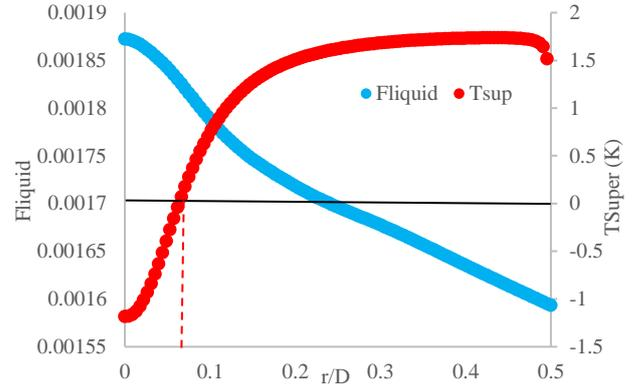
(a) Mist fraction and fluid temperature at fluid vicinity adjacent to heater
