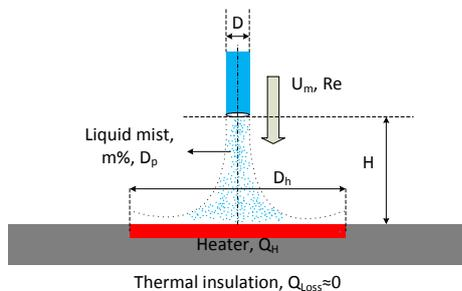
Figure 1. Schematic of investigated round jet and key dimensions
