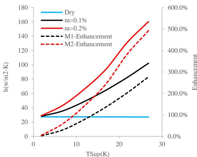
Figure 4. Heat transfer coefficient of dry and mist jet impingement at  $Re=400$
